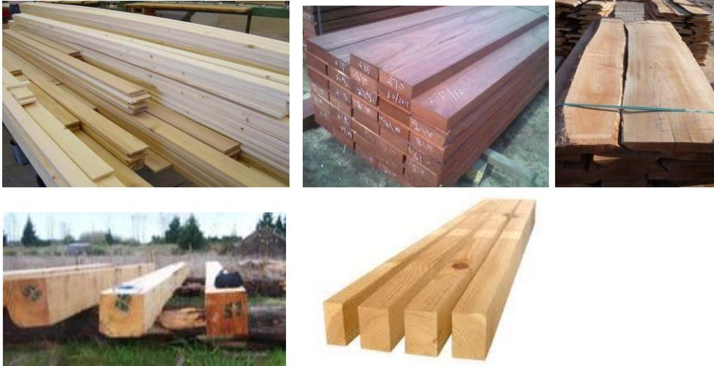
Picture 5,6,7,8 & 9: Sawn Timber/Lumber (pieces of logs)/ Large Scantling and Squares LSS
