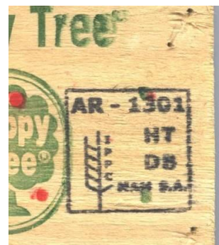
Figure 3 6 – Orientation of information does not match the examples in Annex 2 of ISPM 15. Information included within the borders of the mark exceeds the requirements.
