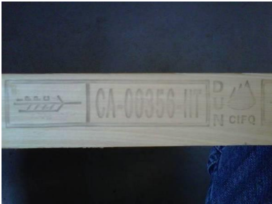
Image 1 5 – Mark matches example 6 of Annex 2 of ISPM 15. Additional information included outside the borders of the mark.
