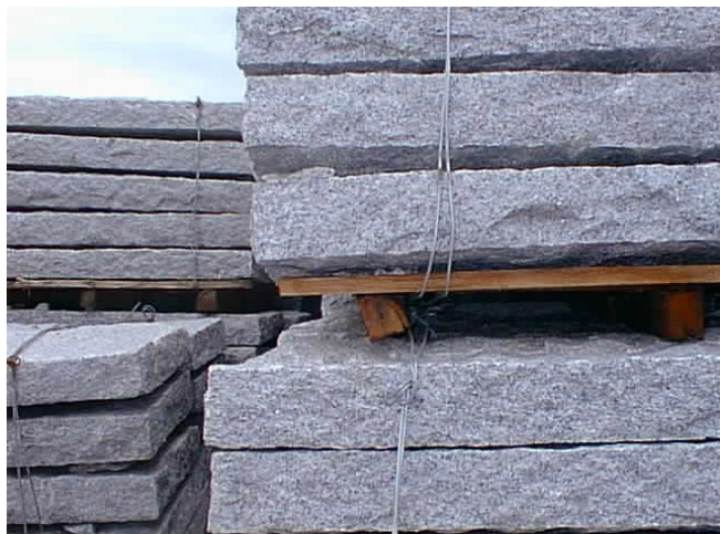
Image 5 - Dunnage attached to stone shipments
