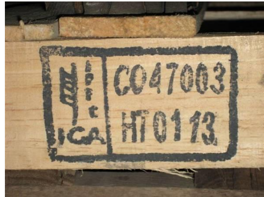
Image 2 6 – Information beyond what is prescribed in Annex 2 of ISPM 15 contained within the borders of the mark.
