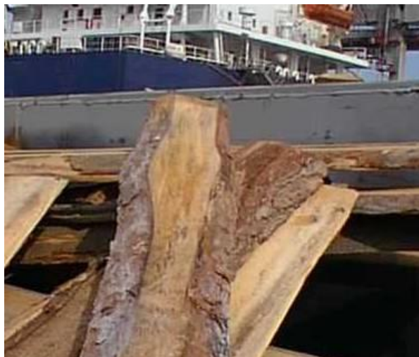
Image 6 - Bark exceeds tolerances. This ship borne dunnage does not comply.
