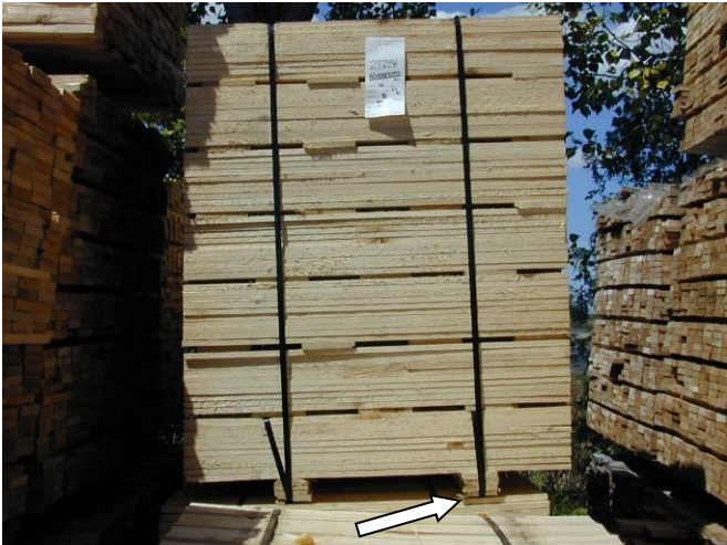
Image 2 - Dunnage used in sawn wood shipments
