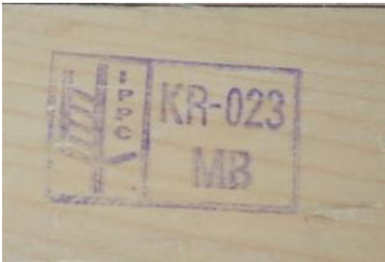
Image 3 6 – Mark matches example 1 of Annex 2 of ISPM 15.
