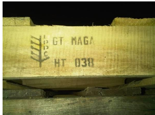
Image 4 6 – Mark does not contain the required borders.
