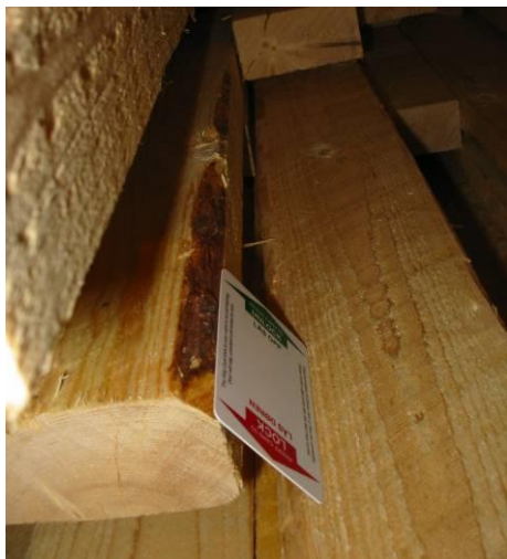
Image 5 - Bark on the edge is wider than 3 cm and the piece is greater than 50 cm 2 . The bark must be removed or the piece may not be used in wood packaging material.
